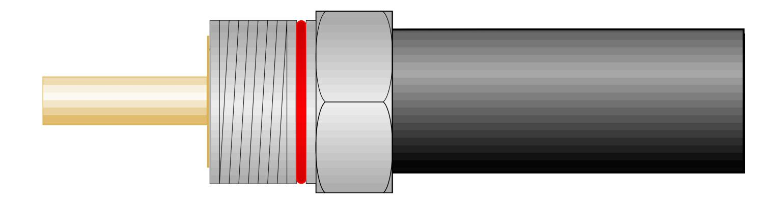
Squarely trim the centre conductor so that 7mm is protruding from the locking nut, if necessary file flat then ensure any debris is cleaned away.
