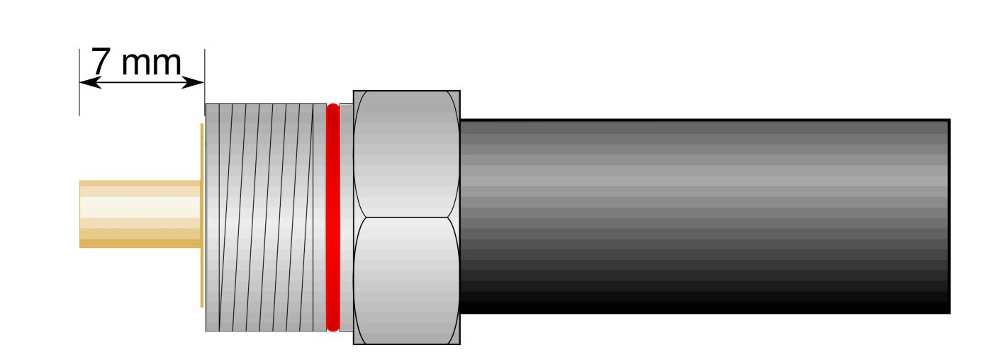
With two spanners, hold the locking nut stationary and tighten the connector body onto the locking nut
